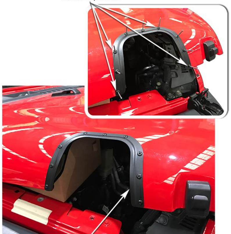
Installed Hood Bezel
